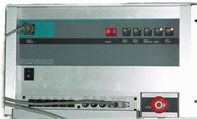
Figura 2.4: Controlador CRS Robotics C 550C.
