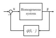
Figure 1. Lur'e-like system with a homogeneous block in the forward path.
