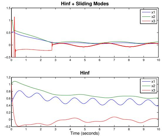
Fig. 5. Sliding modes with  $H_\infty$  and  $H_\infty$  only
