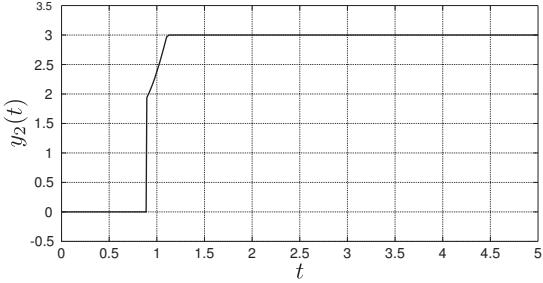
Fig. 8. Time history of  $y_2$  for (16) with the parameters given in Table I, regulated by regularized controller (19) and subject to the perturbation  $d(t) = 5 \sin(t)$ . The finite-time convergence of  $y_2$  to  $y_d$  is still verified.
