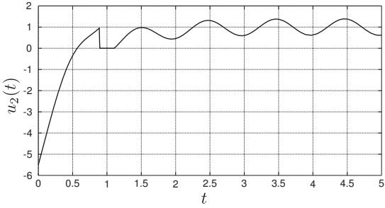
Fig. 9. Regularized control (19) for (16) with the parameters given in Table I and subject to the perturbation  $d(t) = 5 \sin(t)$ .
