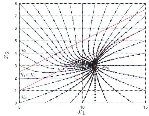
Fig. 4. Phase plane of (16) with the parameters given in Table I. Regulation is achieved with the controller  $u_2 \in \partial\Psi_S(y_2)$ .
