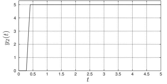
Fig. 7. Finite-time convergence of the output of regulated plant (1) with parameters (18).
