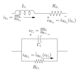
Fig. 1. Current controlled resistors in series with inductors and voltage controlled resistors in parallel with capacitors
