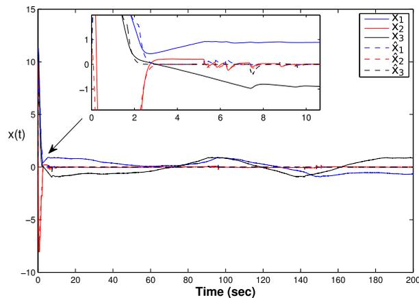
Figure 9. Actual states and estimated states for Example 2 with  $c = 2$ .
