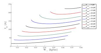
Fig. 3. Steady-state analysis of the system performance in different load conditions
